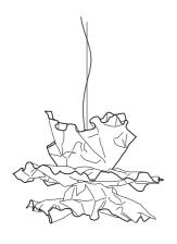
Sheet aluminum with leaf gilded surface by hand or coated with matt colours. Formed by hand. Each piece is unique. 2 x LED approx. 12 W, Ra 90 warm white, 3000 K, integrated, ballasts mounted on luminaire, Colour of cable transparent Pendulum length standard 2.5 m
