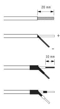
[A] Assembly of the luminaire cable
