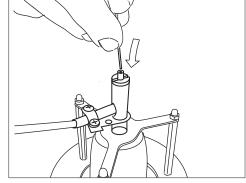
Remove a 3 cm section from the outer covering of the lamp cord and strip about 1 cm of the ends of phase, neutral and protection earth wire. Fit wire end-sleeves.
