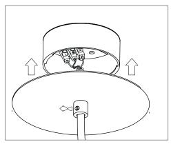
Put the lustre terminal into the canopy. Close the canopy while turning the cover clockwise.
